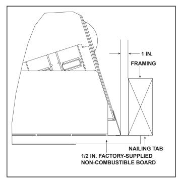
Figure 13.2 Front Side Finishing Detail
